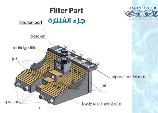
The filtering part includes one prefilter baskets + cover for connection with water vacuum cleaner; one carttage filter; one skimmer; nozzle; LED lights 6x18W 12000K; LED spotlight; LED lighting of hydro massage nozzles; hydro massage (ten hydro massage nozzles); blower (air massage); switch buttons of counter-swimming, blower, nozzles' lighting and LED spotlight.
